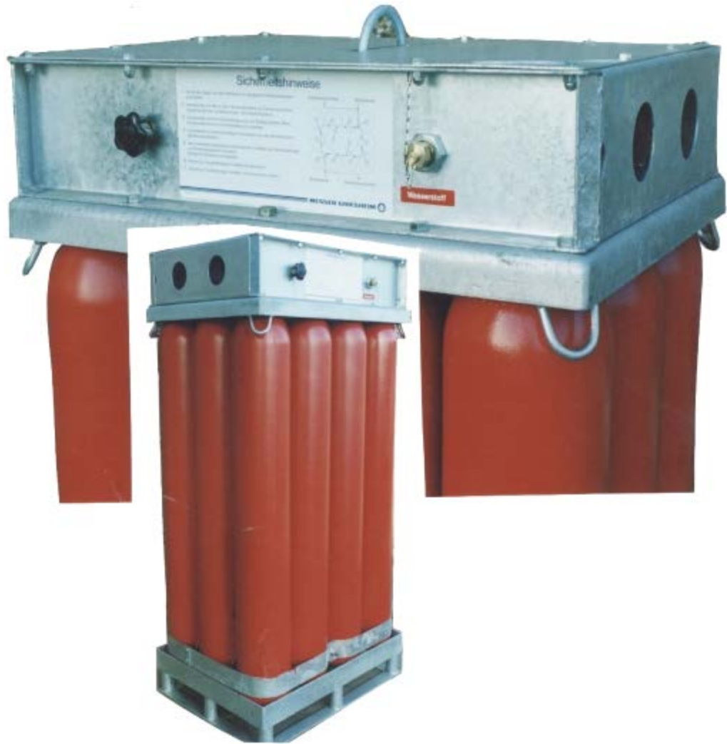
Figure D.1 : Modern hydrogen bundle design, according to EN 13769, containing 12 cylinders with 50 ltr. water capacity / 200 bar filling pressure each
