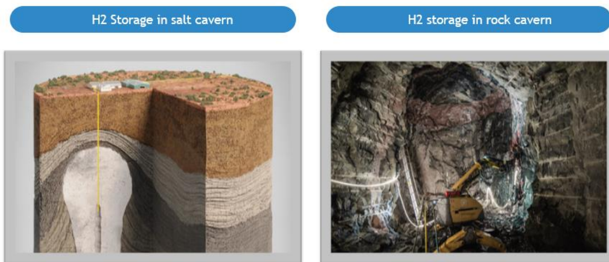
Figure 3:a). H 2 Storage in a salt cavern, b). H 2 storage in rock cavern (Source: Google)
